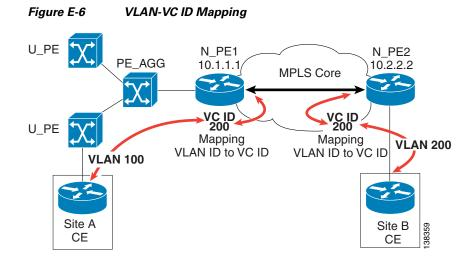
The VLAN IDs allocated and used at each access domain do not have to be the same.
